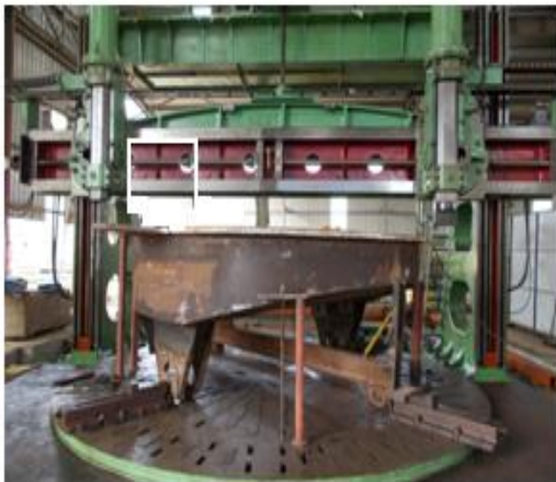
Fig. 1 structure of vertical turning lathe
