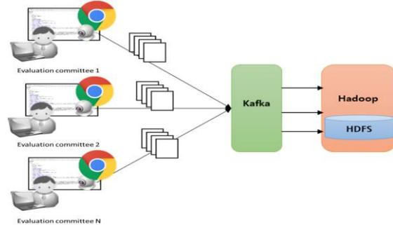
Figure 1 Design of a collection system for the Absent Detection Rate detection system
