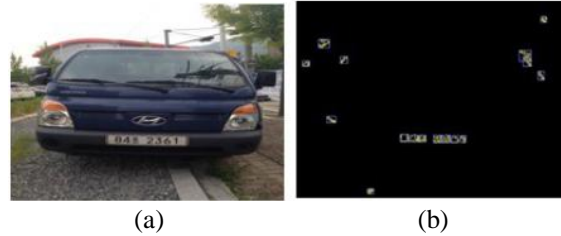
Figure 5. License plate-like contour extraction image (a) Original image (b) Outline extraction image
