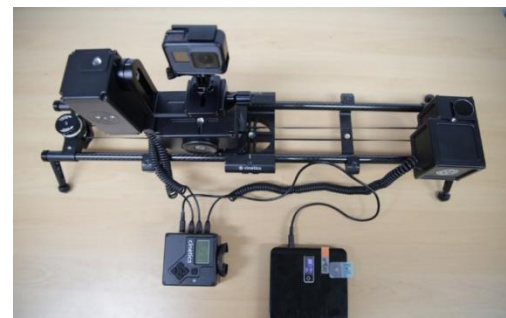
Figure 3. 3DOF – Pan, Tilt, Slide controller
