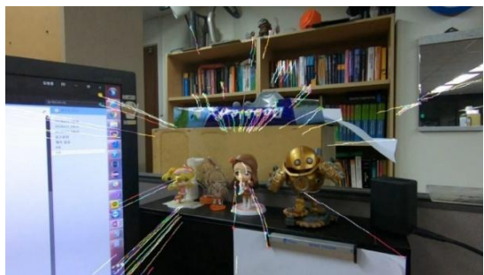
Figure 5. Pyramid Lucas-Kanade method applied video
