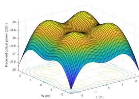
Figure 5. Received signal strength for 4-LEDseach position
