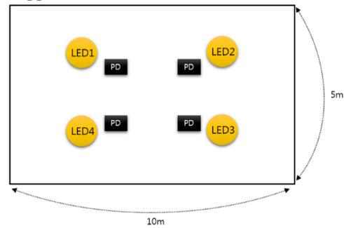
Figure 4. Indirect light source interference model floor plan
