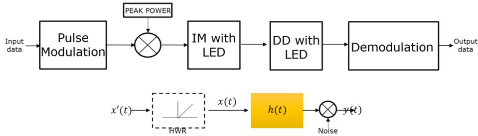
Figure 1. VLC system model
