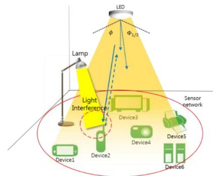
Figure 2. Iot network interference scenario
