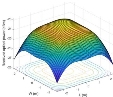
**Figure 6. Received signal strength for 5-LEDs each position**
