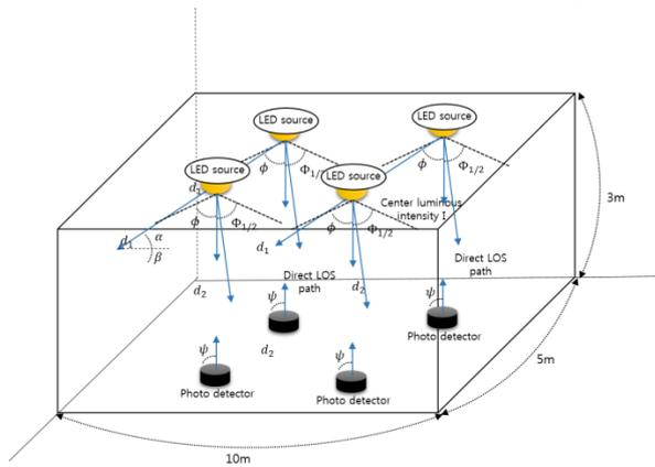
Figure 3. Indirect light source interference model design
