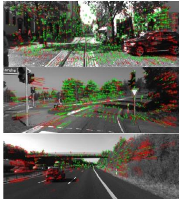
Figure 2. Results of inlier (green) and outlier (red) determination.
