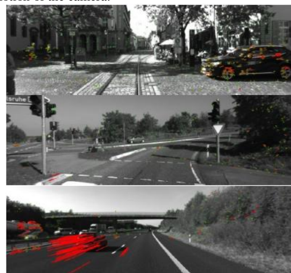
Figure 3. Results of compensating for optical flow using estimated camera motion.
