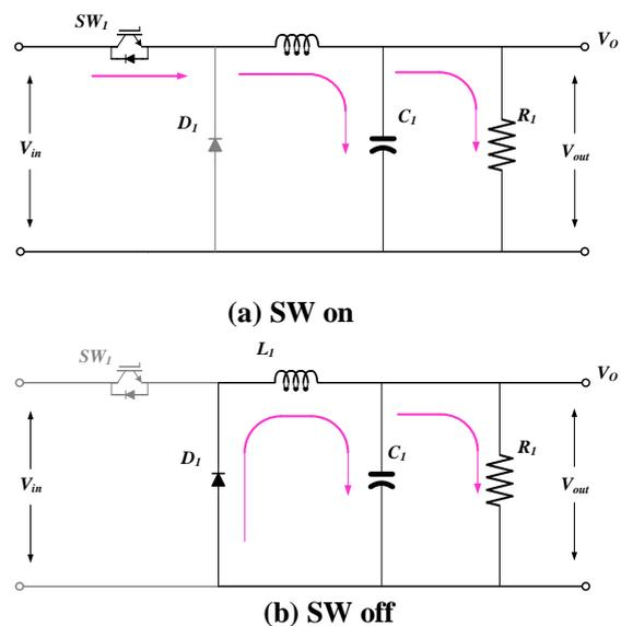
**Figure 1. Conventional buck converter**
