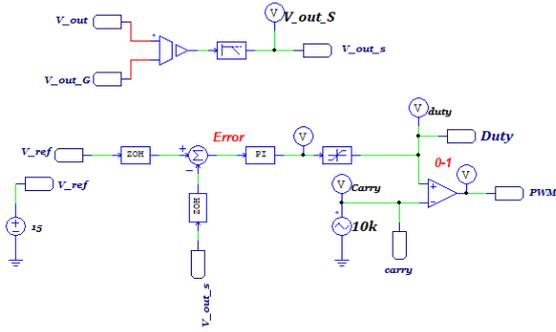
Figure. 7 Simulation of Conventional buck converter and output voltage sensing method
