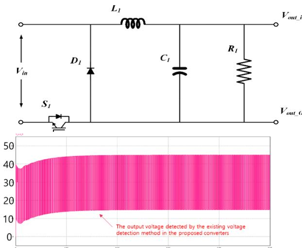
Fig. 9 Modified buck Converters and Waveform of output voltage
