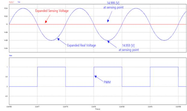
**Figure 6. The output voltage waveform detected by the proposed method**
