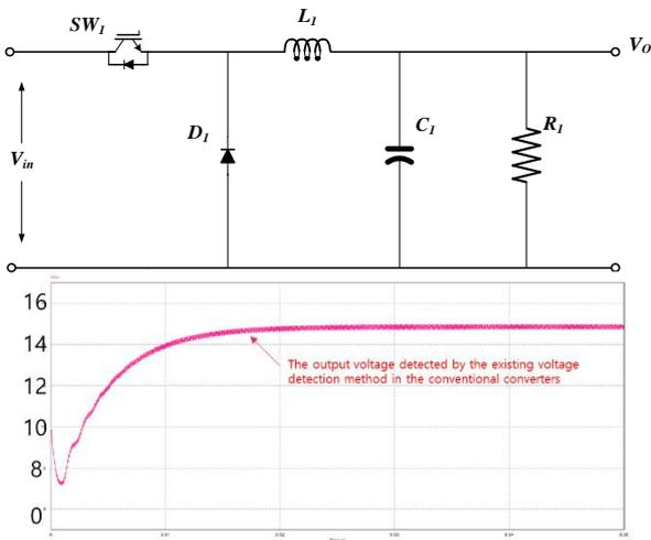
Fig. 8 Conventional Buck Converters and Waveform of output voltage
