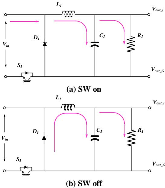
Figure 3. Modified buck converter and operation
