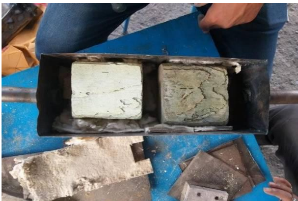
“Fig.” 8 Both ceramic block placed in a casing
