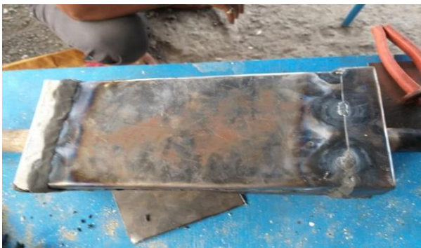
““Fig.” 9 Fabricated Catalytic converter having inlet and outlet manifold
