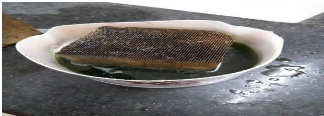
“Fig.” 2 Monolith ceramic block is dipped into HCL Solution
