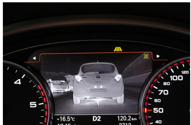
Fig. 1. Configuration of automotive night vision system (Audi A8)
