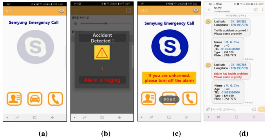
Figure 7. Screenshot of the Smart-phone Application for the Proposed System (a) Initial Screen of the Proposed App, including Registration Icon, (b) Screenshot of Alarm ringing due to Emergency Situation, (c) How to Turn-off Alarm, (d) Emergency Relief Letter to family or friends (Pre-registered phone number)
