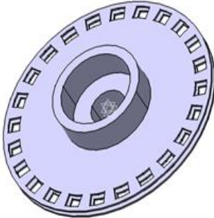
(b) Torque sensor disk (26 grooves) of model 2
