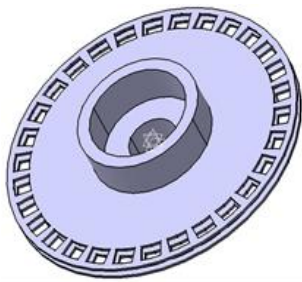
(a) Torque sensor disk (31 grooves) of model 1
