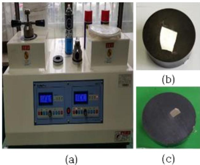
**Fig. 1** Mounting press and specimens
