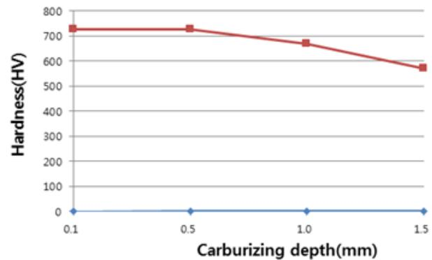
**Fig. 3** The carburized hardness distributions of alloy steel.
