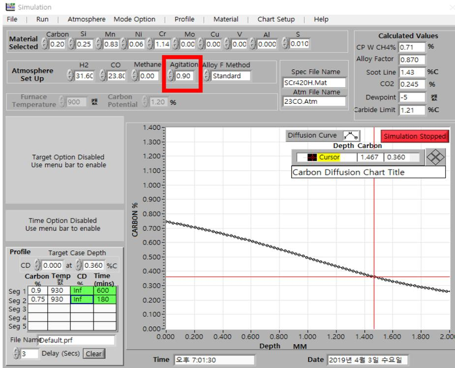
Fig. 7 (b) Carburized amount and carburizing depth from simulation data.
