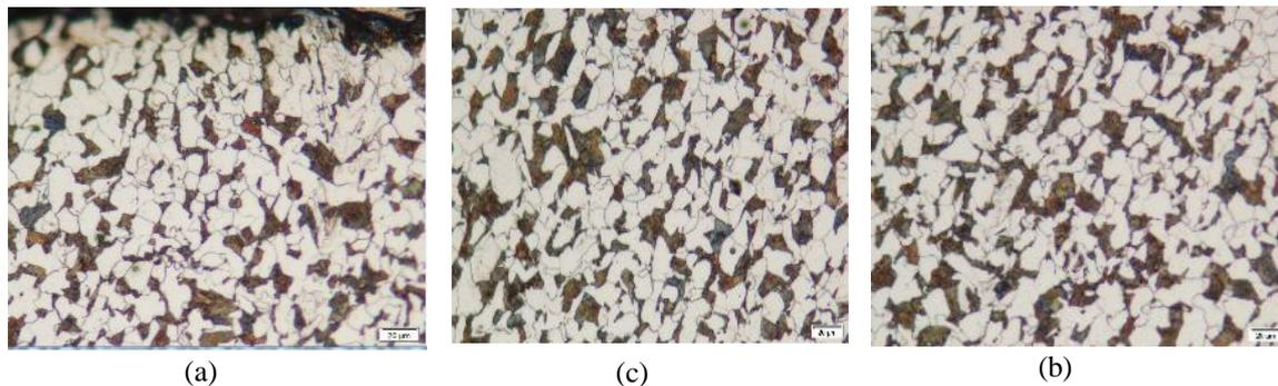
**Fig. 4.** Optical microscope photographs : before carburizing of alloy steel[x500].
