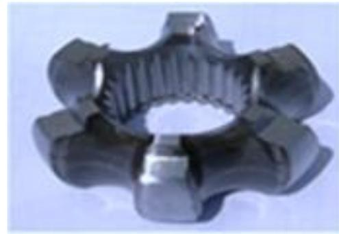
**Fig. 2** Carburized inner race.
