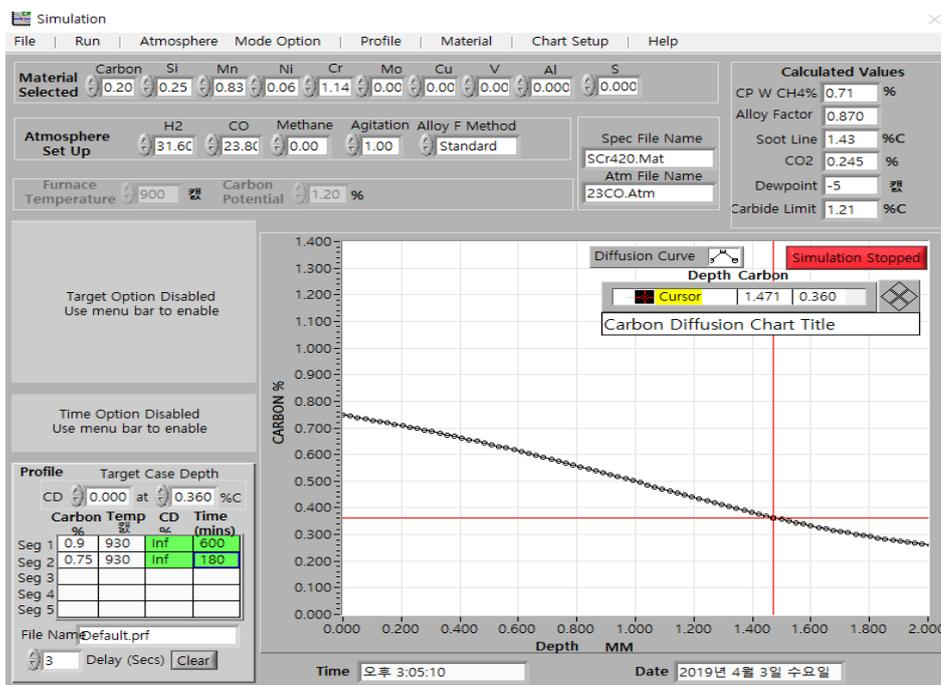
Fig. 7 (a) Actual carburization amount and carburization depth.
