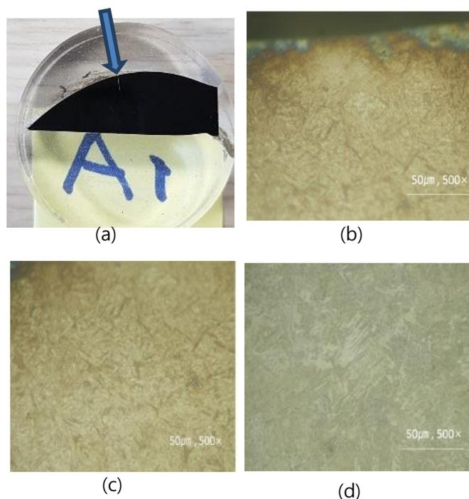
**Fig. 5** Optical microscope photographs : Carburized alloy steel[x500].
