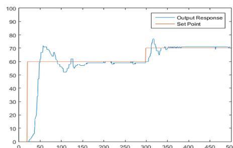
Figure10. SMC control action results on experimental setup with changing set point
