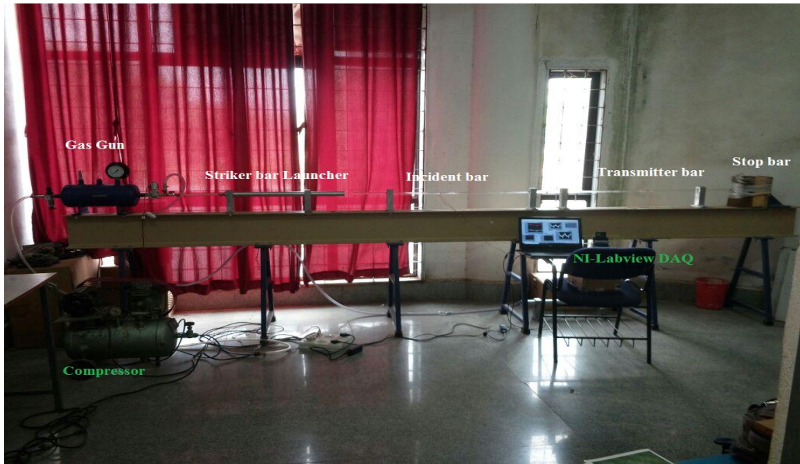
Figure 3 Photograph of a Polymeric SHPB Setup
