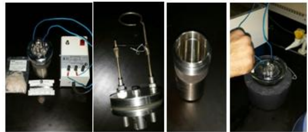
Figure 9. Oxygen Bomb Vessel for Determining Heat Content
