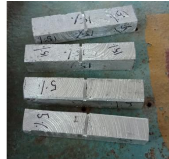
Fig: 4-Specimens Prepared for Charpy Impact test
