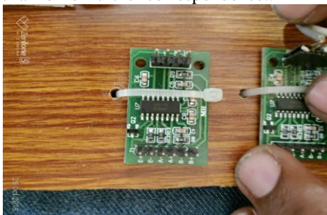
Figure 2: HX711 Strain gauge drivers(x2)
