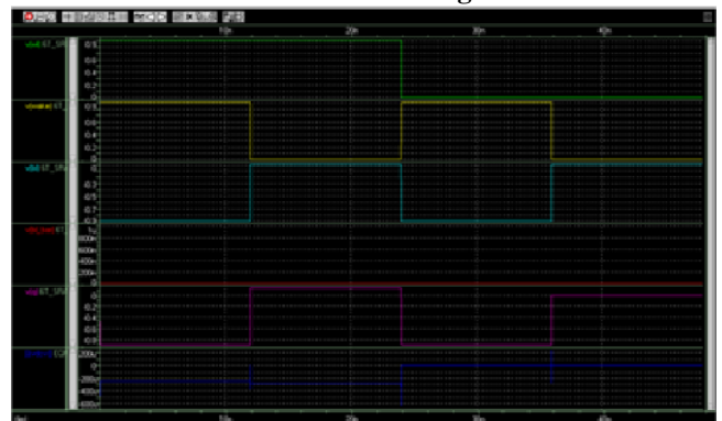
Figure 9.Performance of Write operation of the 6T-SRAM-AAM design
