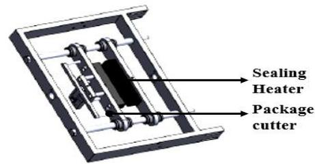
Figure 4. Sealing unit of the VFSS system
