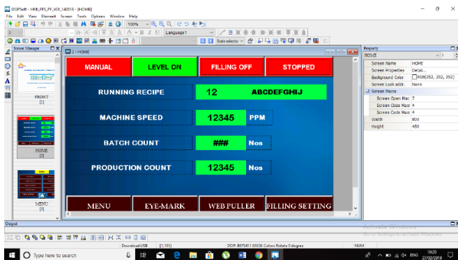
Figure 6. HMI menu for monitoring the overall packing process
