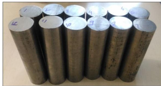
Figure No. 2 - Work piece Material AISI 316
