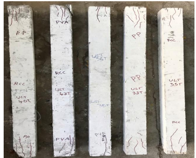
Fig.5. Crack pattern of column
