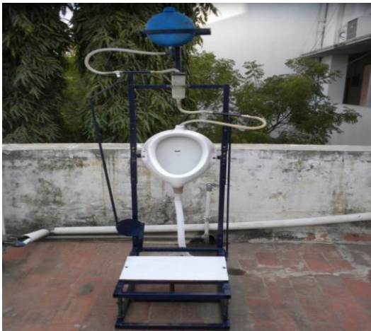
Fig.32 Fabricated model of Automatic Urinal Flushing System
