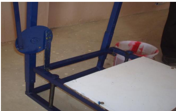
Fig.33 Clock wise rotation of Rocker arm, Opens the inlet valve
