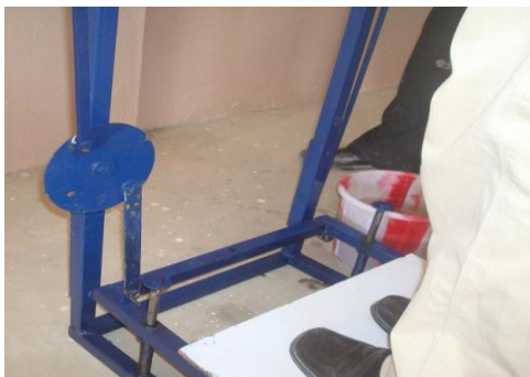
Fig.34 Anti clock wise rotation of rocker arm -opens the outlet valve
