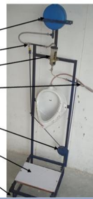
Fig.31 Components of Automatic flush system
