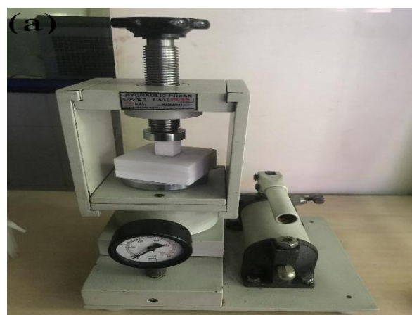
Fig.2(a): Hydraulic press used to press the mould
