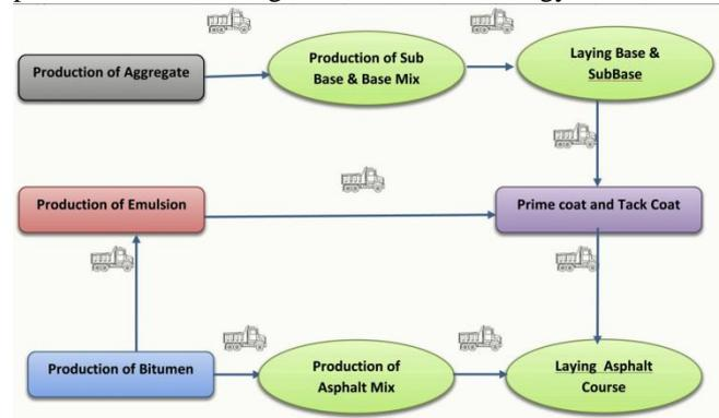
Fig. 3: Process of Construction of Asphaltic Pavement
