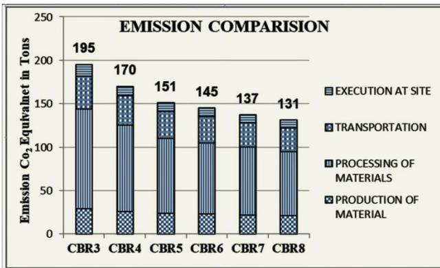
**Fig. 10:** Emission of CO<sub>2</sub> equivalent in tons for various CBR for a pavement of 1km length , 7.00 m width.
