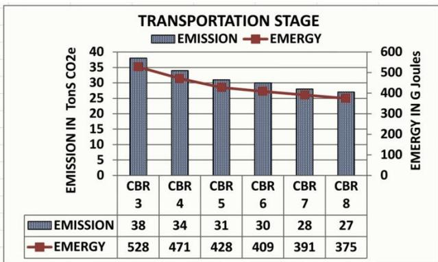
Fig. 14:Energy consumption and the emission transportation stage
