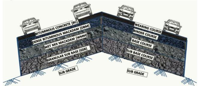
Fig. 4:Cross section of a flexible pavement
