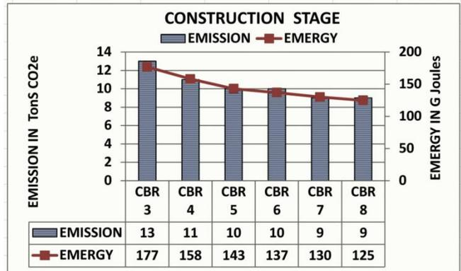
Fig. 15: Energy consumption and the emission construction stage.
