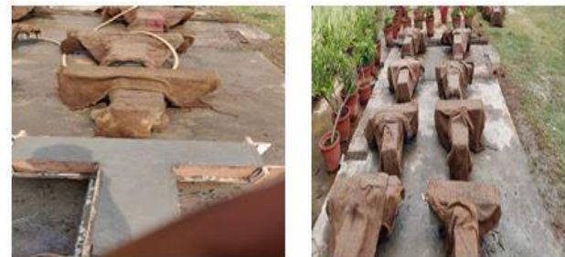
Figure 1: (a) Casted specimens , (b) Curing of specimens
