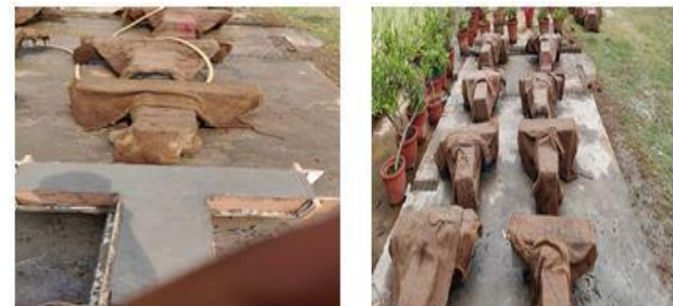
Figure 1: (a) Casted specimens , (b) Curing of specimens
