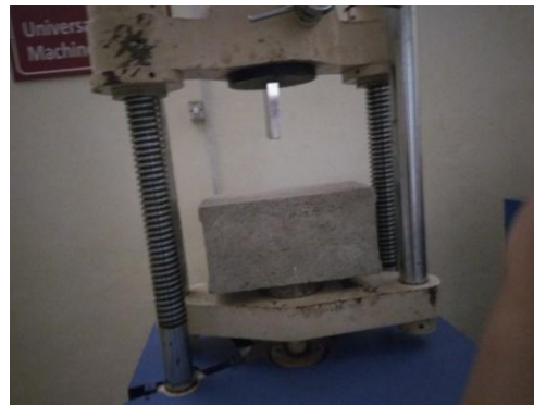
Figure 5: Flexure Test of Concrete Block
