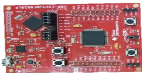
Fig. 2. Master controller launch pad Table 2. Features of MSP430G2553
