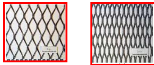
fig1.Hardware samples used in ferrocement.
