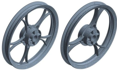
Figure 5. Meshing for V curved shape with pad with 3 and 5 spokes
