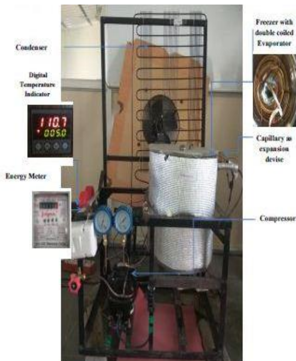
Fig.1 Vapour compression Test Rig
