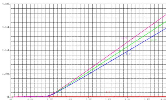
Fig. 3  $I_c$  vs  $V_s$  characteristic at constant  $V_g$
