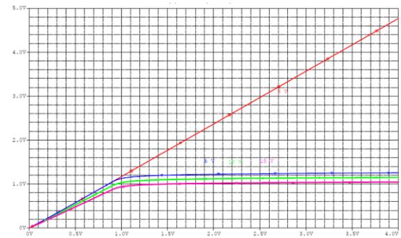
Fig. 4  $V_{ce}$  vs  $V_s$  characteristic at constant  $V_g$
