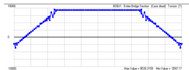
Variation of Torsion along the along the 120 degree curved bridge with no skewness
