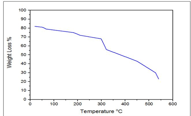
**Figure 1: TGA curve for PPVA-SGO membrane**
