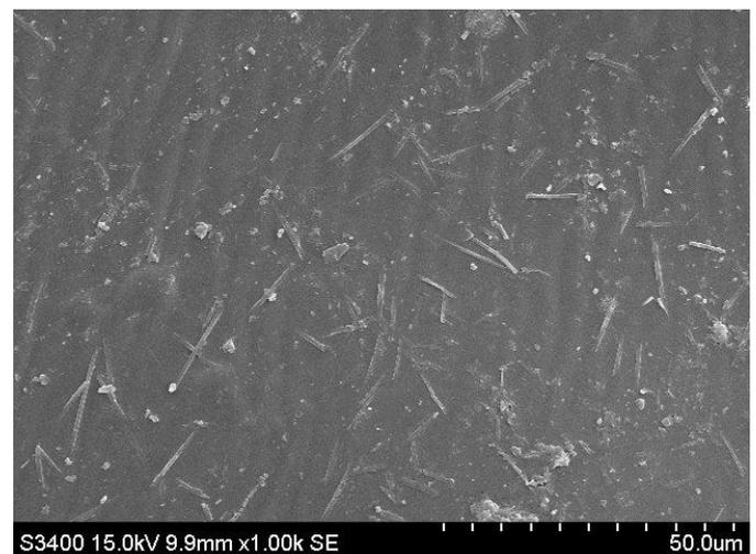
**Figure 2: SEM Image for PPVA-SGO membrane**
