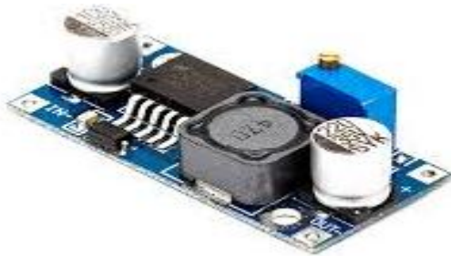
Figure 6. Step down voltage regulator
