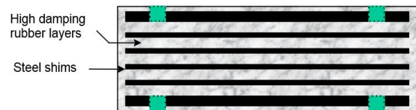
Fig. 4. Cross section of high damping rubber bearings
