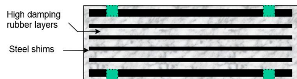
Fig. 4. Cross section of high damping rubber bearings
