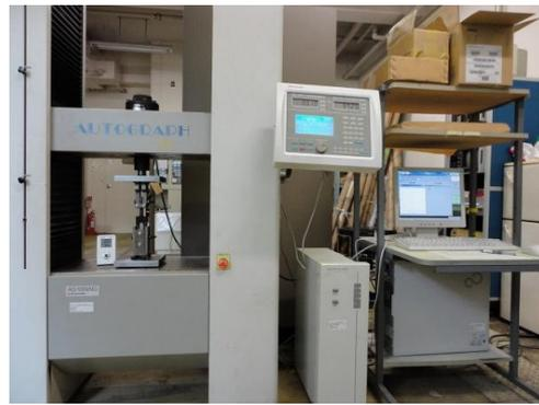
Fig. 4: The testing machine for lap shear tests.
