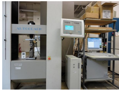
Fig. 4: The testing machine for lap shear tests.
