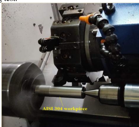
Figure 2 Experimental set for machining test
