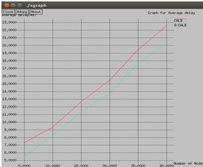
**Fig. 6. No. of nodes Vs. average delay**
