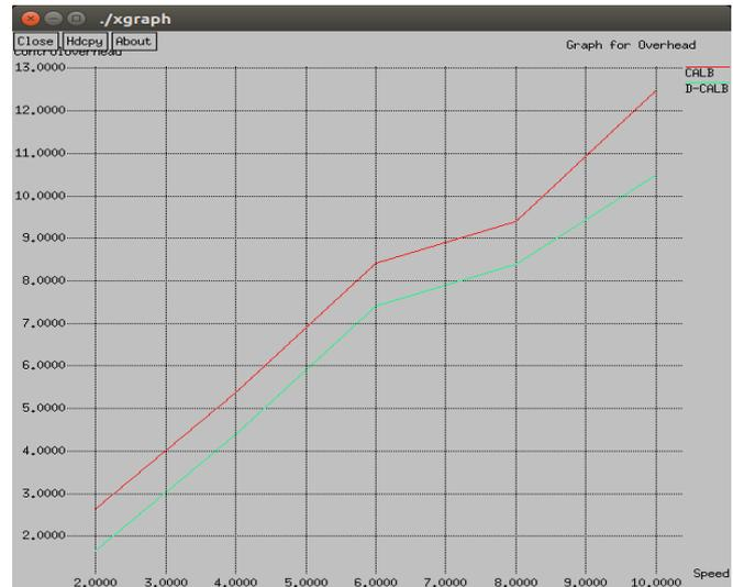
**Fig. 13. Varying speed vs. Normalized routing overhead**
