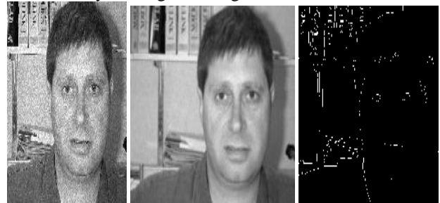
Figure 5 (i) Distorted Image (ii) Smooth image and (iii) Region Image Fig 5 (i) Represents the distorted image means noises presented in the uploaded image. 5(ii) shows that the filtered image means to remove the interference in Noisy image and output produces the smooth image. 5(iii) Region calculated by Sobel method and maximum values fetch in the smooth image.
