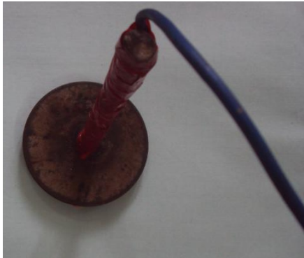
Figure 12: Circular disc probe of diameter 75mm
