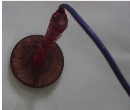
Figure 12: Circular disc probe of diameter 75mm
