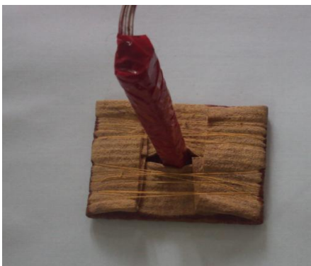
Figure 13: Rectangular probe of size 105mm x 75mm
