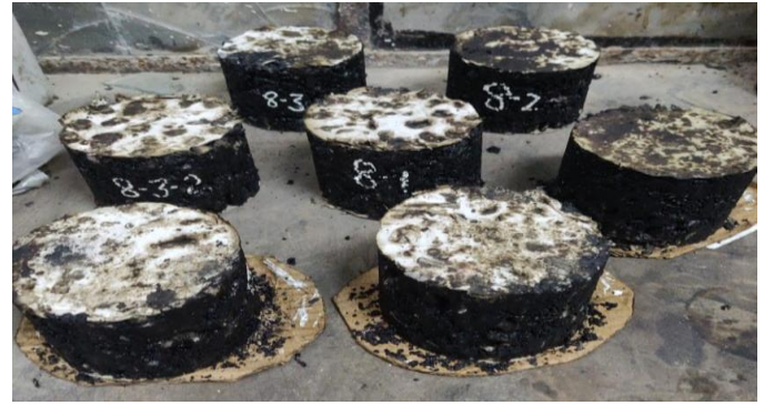
Fig.2: Samples were prepared at different binder content
