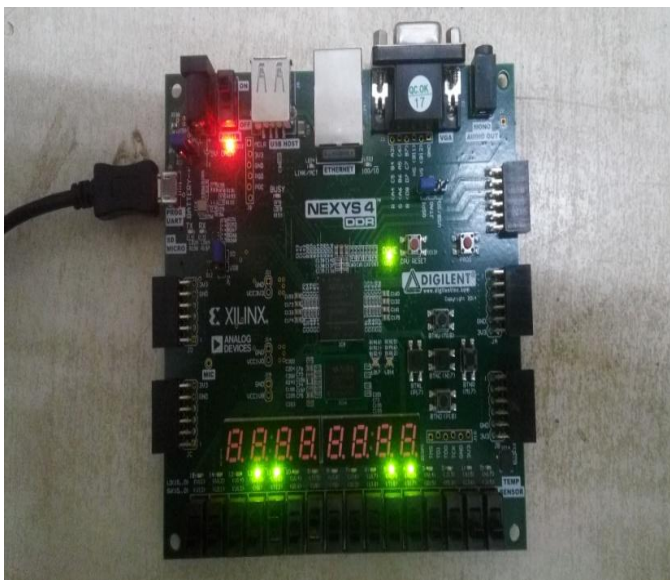
Fig7. Hardware implementation on Artix 7 FPGA for two antenna elements.
