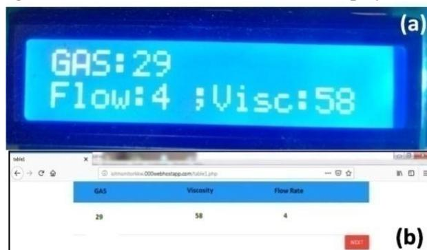
Pre-designed web page depicting observation of gas, viscosity and liquid flow rate.
