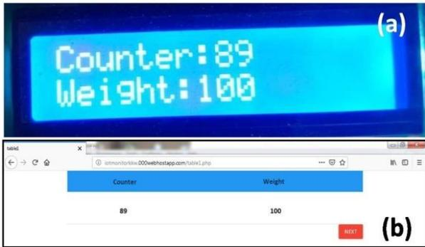
**Fig 4. (a) Real time results shown in LCD display and (b) Counter and weight sensors indicating the observed reading in real time on website.**
