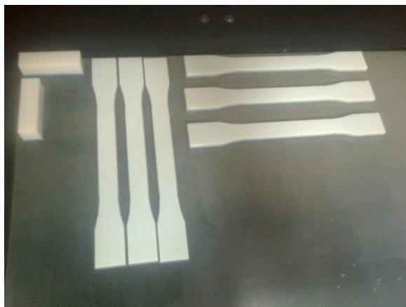
Fig 2 Fabricated Specimen Based on Orientation
