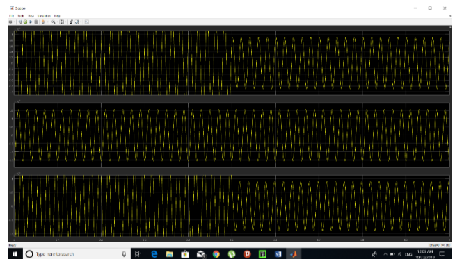
Fig 5: L-G Fault voltage wave form
