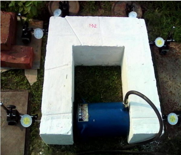
Figure-3 Hydraulic jack & dial gauge arrangement installed for testing the beam column joint specimens
