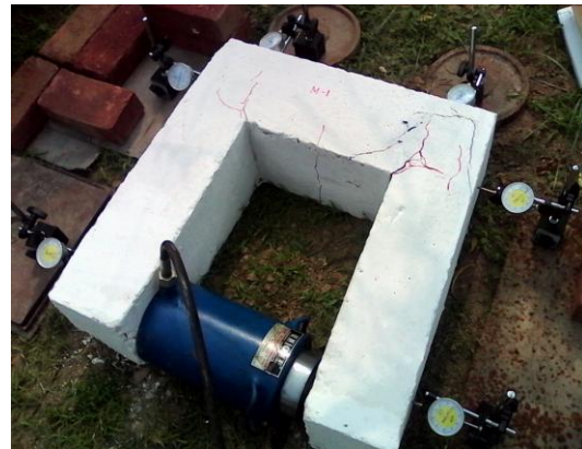
Figure-5 Testing of retrofitted beam column joint
