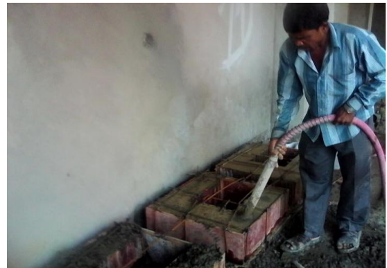
Figure-2 Casting procedure of specimens
