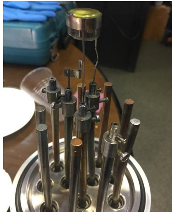
Fig. 2. CdZnS/ZnS (GT) specimen just before mounting the flange to a vacuum chamber
