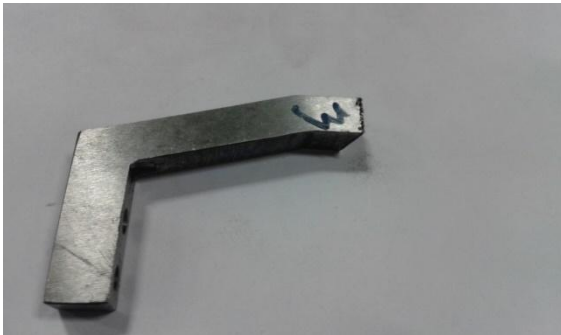
Fig. 4 Component where de-burring operation is not performed
