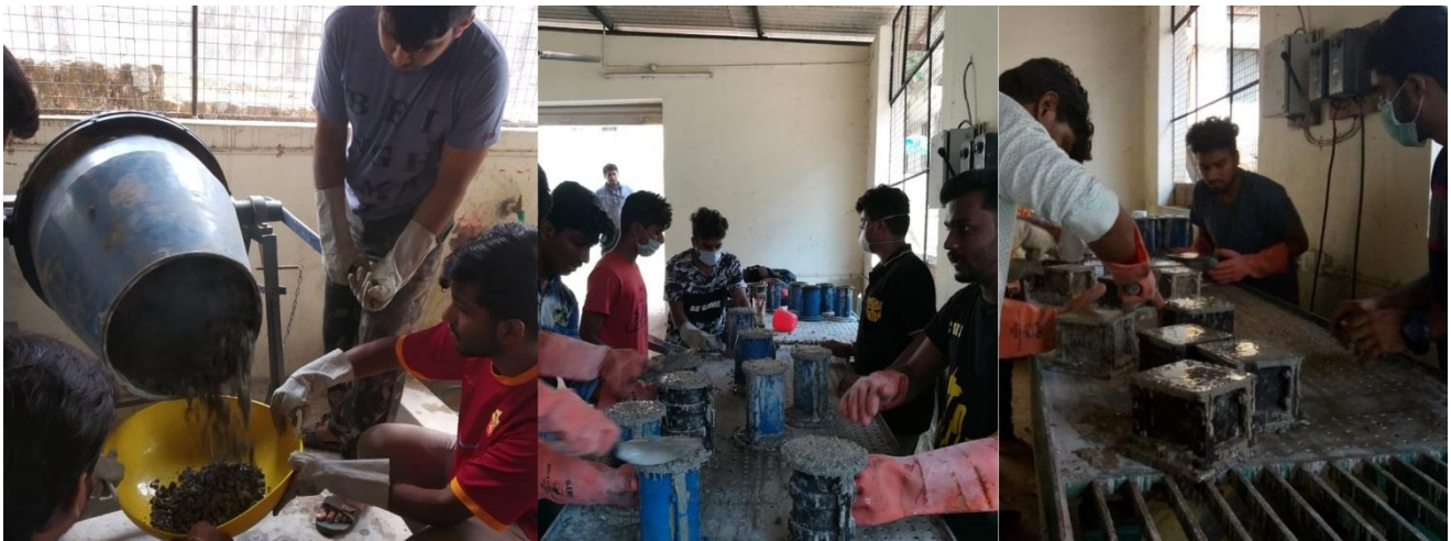
Fig. 1: Mixing of Concrete, Filling the standard molds and Vibratory Compaction for Casting of test specimens
