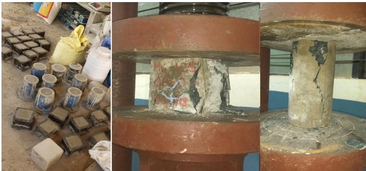
Fig. 2: Air curing in the laboratory, the typical mode of failure of cube and cylinder specimens under compression
