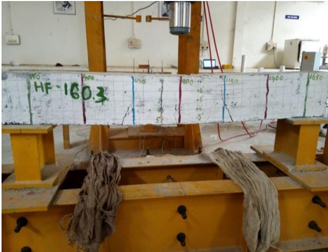
Figure19 After load removal beam regain its normal position
